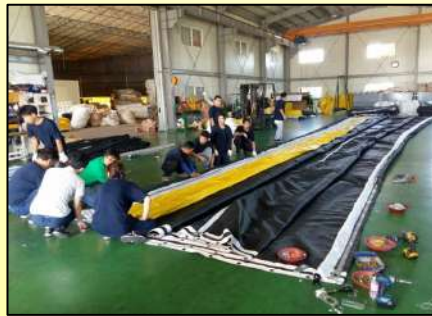
Fabrication of silt curtain
